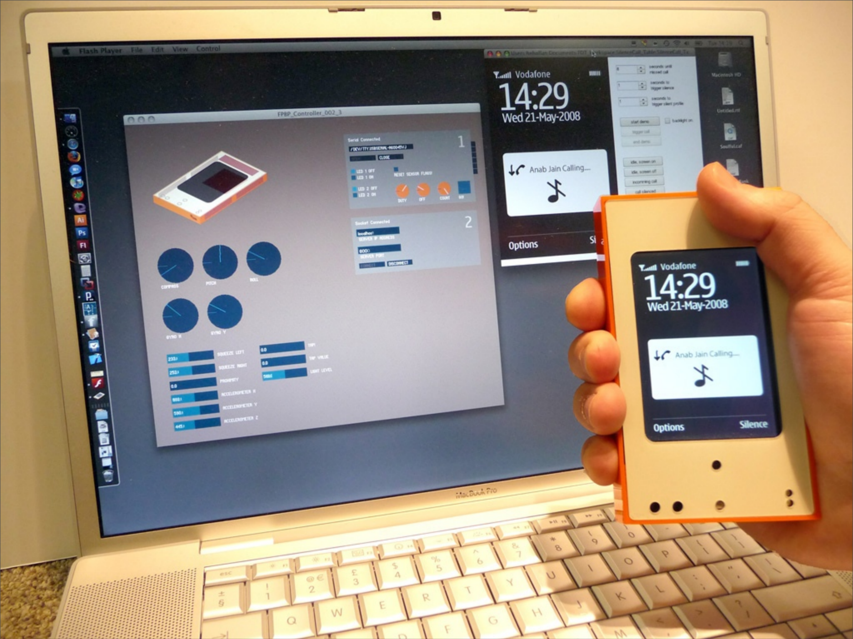
Here's the prototype in action, exploring gestures for silencing a ringing phone. You can see the sensor data displayed on the left of the laptop screen, and the phone UI being sent back to the device on the right.
